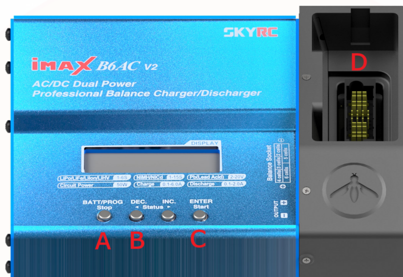
Figure 61: SKYRC Charger/Discharger and Hoverfly Battery Pack
