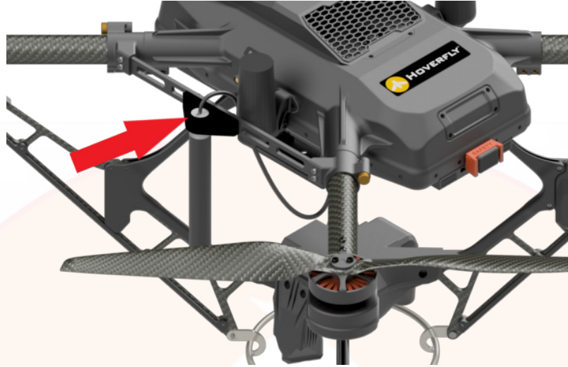
Figure 12: One Octane Antenna Installed on the Spectre Aircraft
