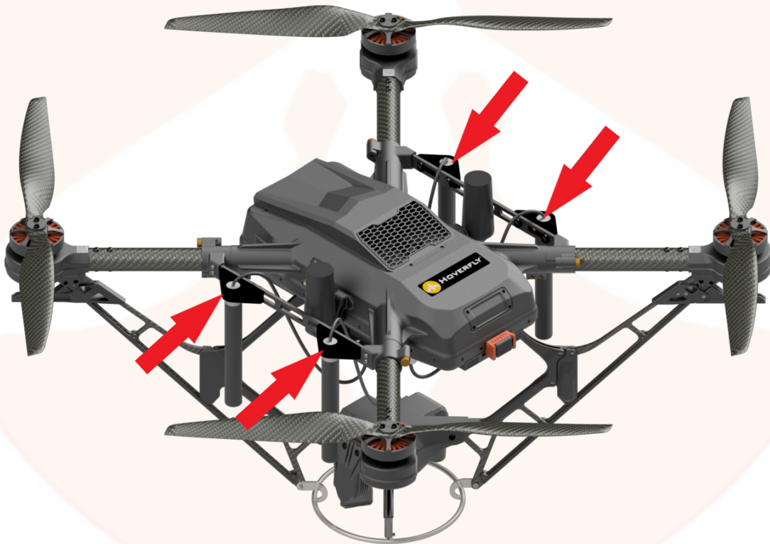
Figure 13: Four Octane Antennas Installed on the Spectre Aircraft
