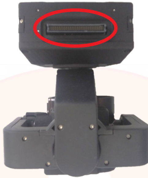
Figure 2: Camera Payload Pogo Pin Connection
