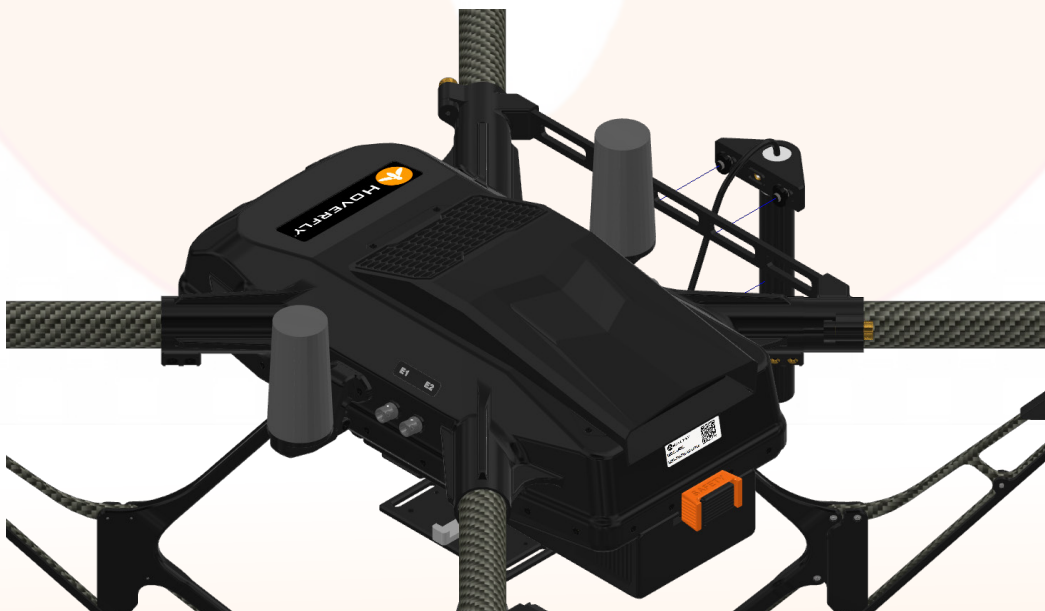
Figure 11: Octane Antenna Installation
