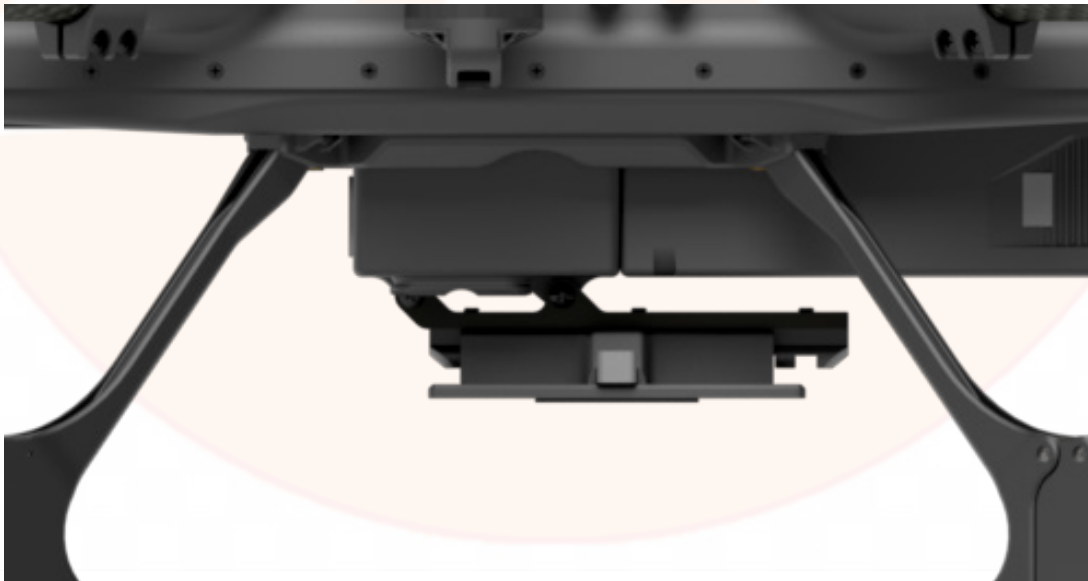
Figure 5: Universal Radio Plate Installed
