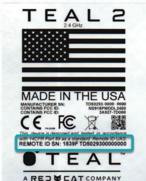
Figure 1 - Example Label, Remote ID Equipped UA
