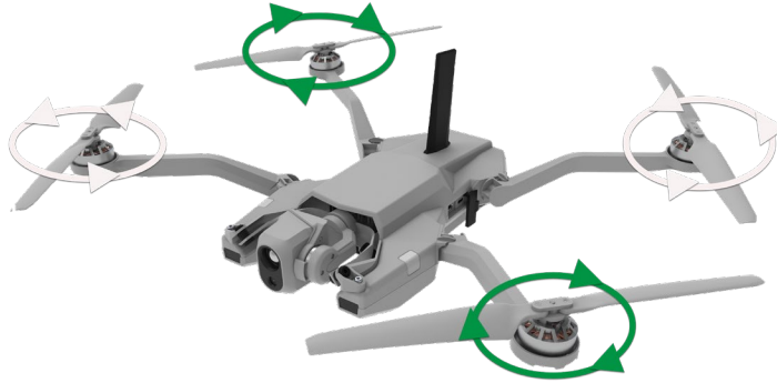
Figure 1 Clockwise and counterclockwise arms and propellers.
