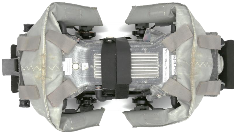
FIGURE 56 - DIODON HP30 FOLDED ON CENTRAL PROTECTIVE FOAM
