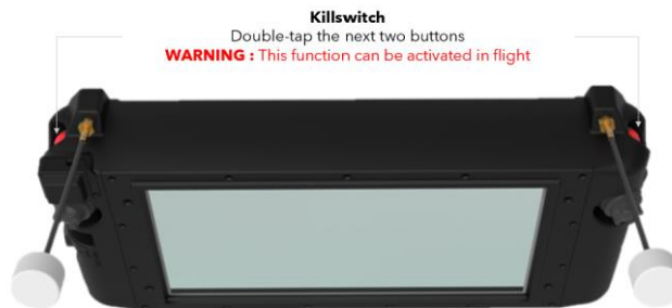
FIGURE 11 - LOCATION OF ENGINE SHUT-OFF BUTTONS
