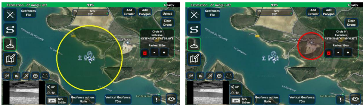
FIGURE 40 - DISPLAY OF GEOFENCE ON THE DIODON HYSTRIX CONTROL INTERFACE
