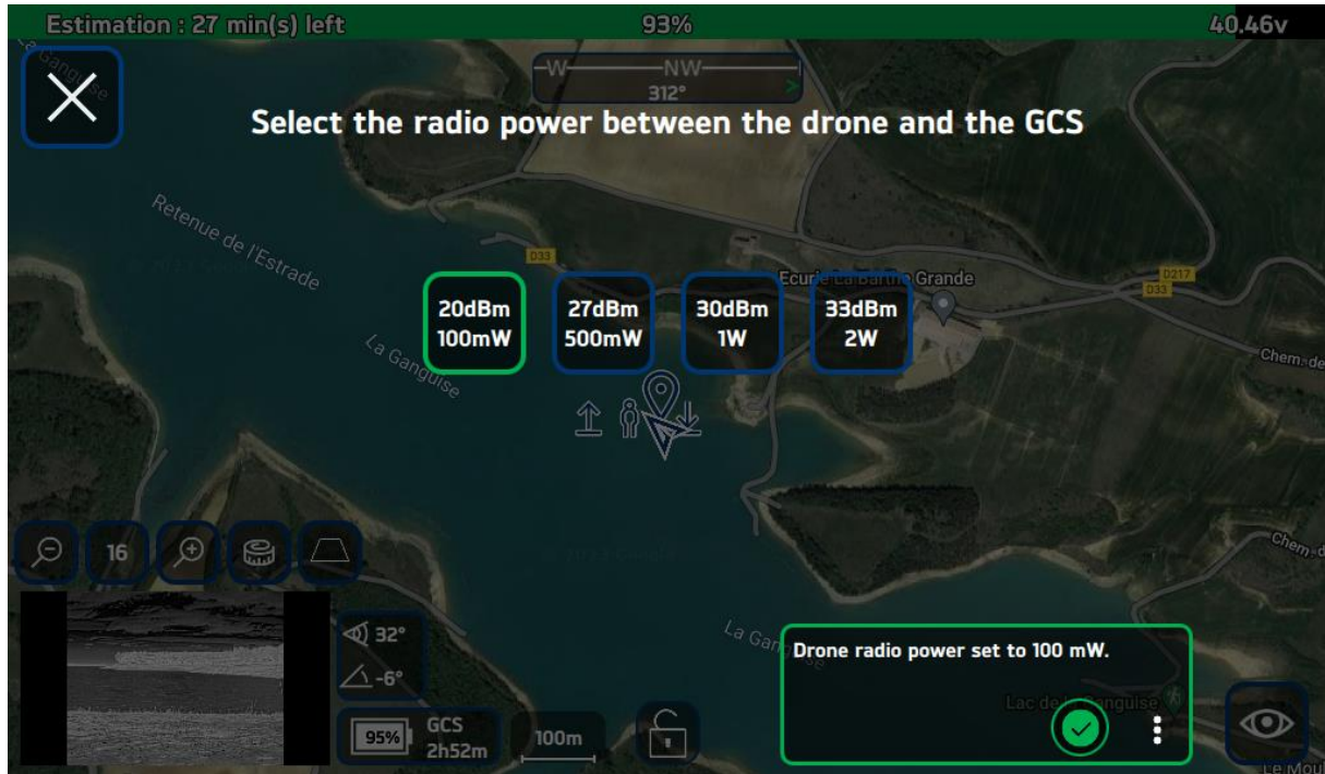
FIGURE 39 - TRANSMIT POWER DISPLAY ON THE DIODON HYSTRIX CONTROL INTERFACE
