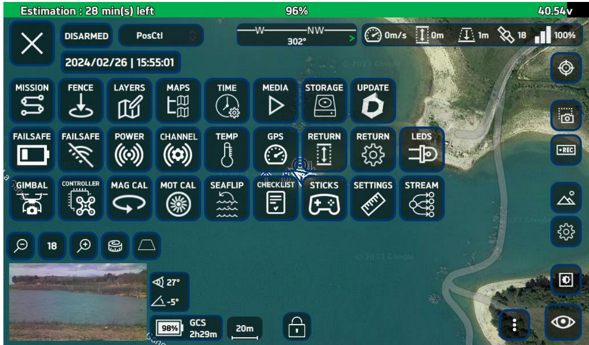
FIGURE 21 - ADVANCED MENU DISPLAY ON THE DIODON HYSTRIX CONTROL INTERFACE
