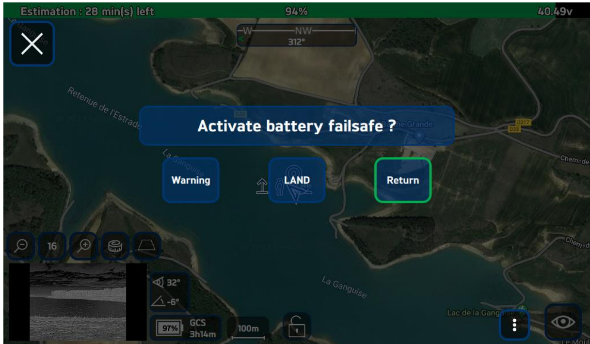
FIGURE 24 - BATTERY FAIL-SAFE SETTING
