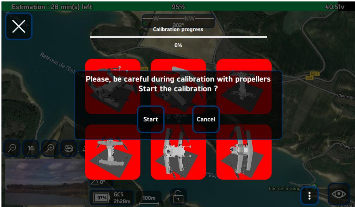
FIGURE 27 - MAGNETOMETER CALIBRATION INTERFACE DISPLAY
