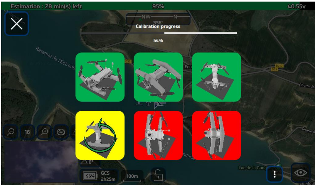
FIGURE 28 - INTERFACE DISPLAY DURING MAGNETOMETER CALIBRATION
