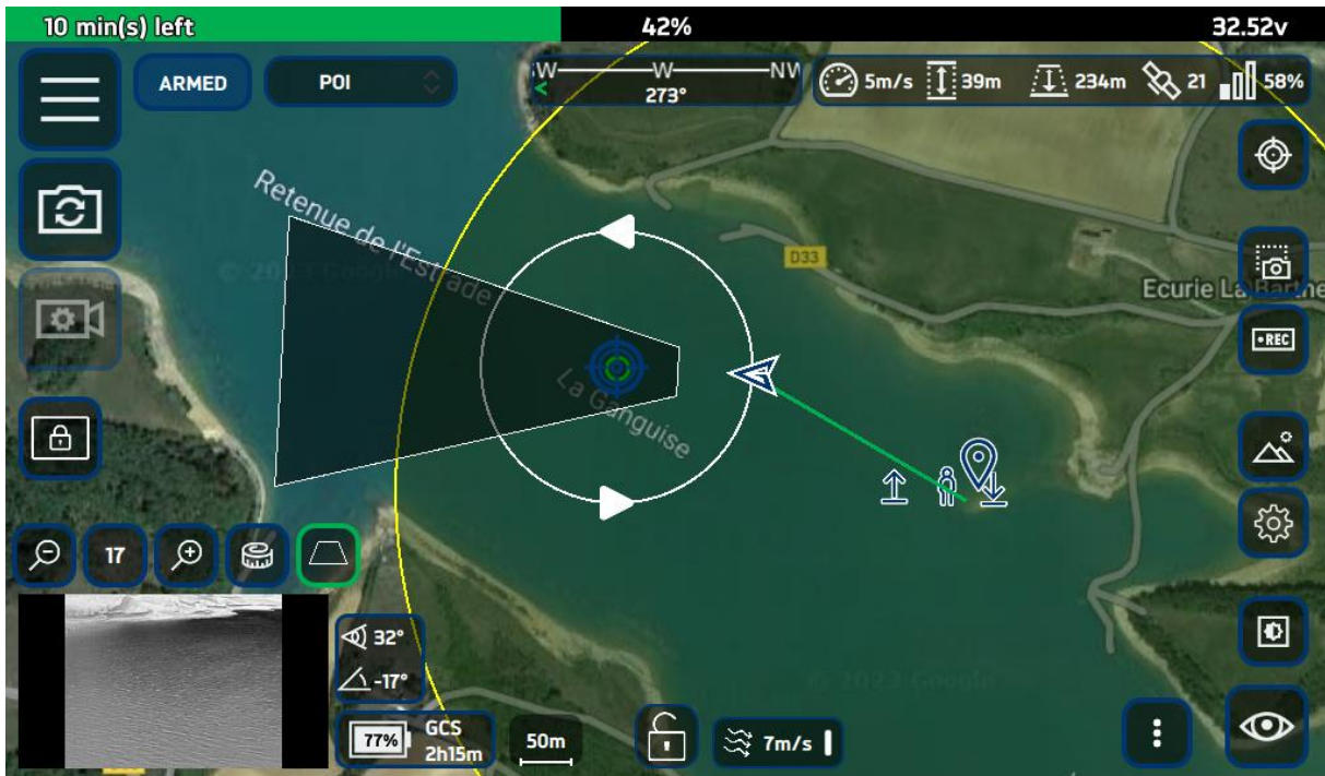
FIGURE 19 - ILLUSTRATION OF ORBIT MODE
