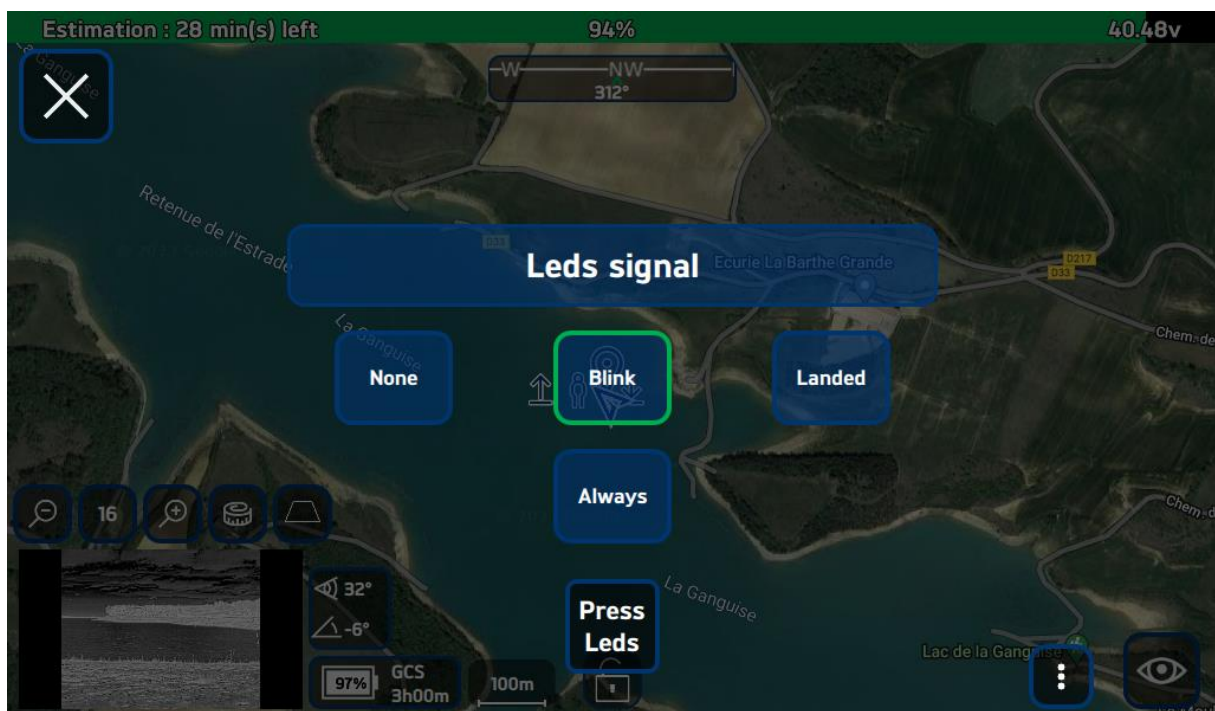
FIGURE 34 - DISPLAY OF LED SETTINGS IN THE HYSTRIX DIODON FLIGHT INTERFACE
