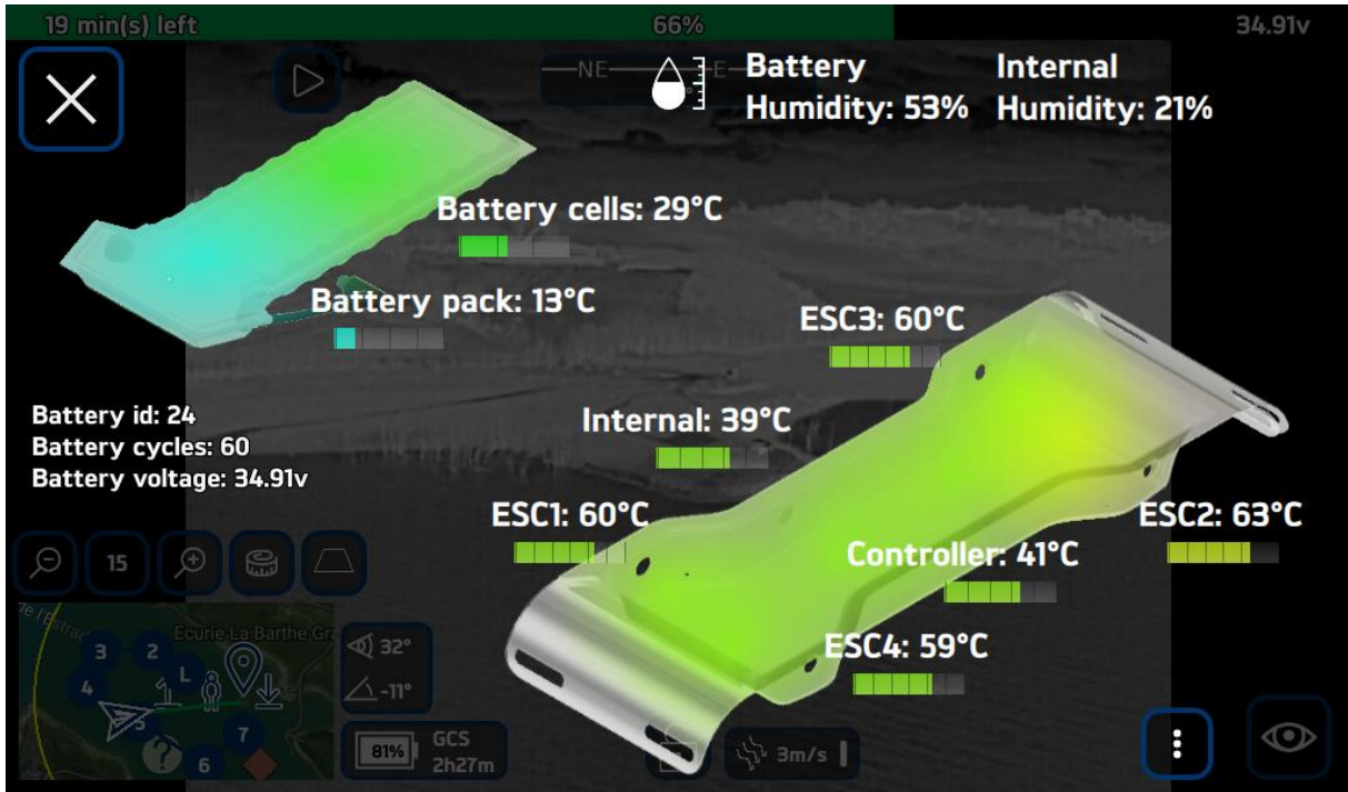
FIGURE 37 - DISPLAY OF INTERNAL TEMPERATURE/HUMIDITY SENSORS ON THE CONTROL INTERFACE
