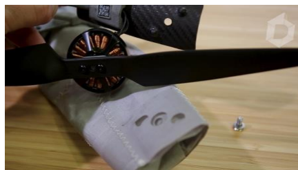
FIGURE 59 - THE DIFFERENT STEPS TO REMOVE THE PROPULSION GROUP
