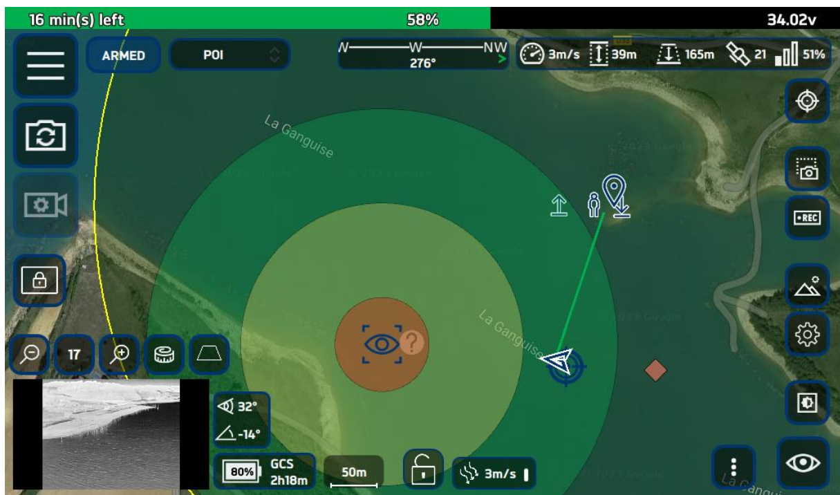
FIGURE 18 - ILLUSTRATION OF GOTO MODE COUPLED WITH LOOK AT FUNCTIONALITY
