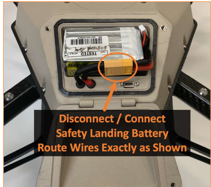
Figure 37. LiveSky Safety Battery Replacement
