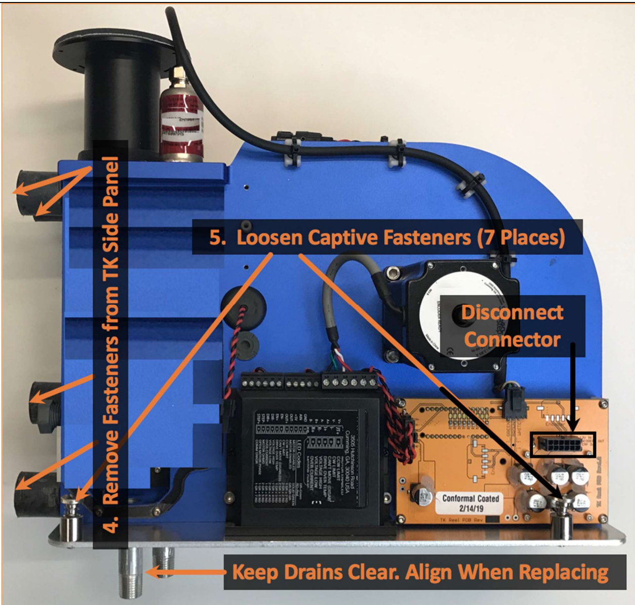
Figure 41. Fasteners on Tether Reel Assembly
