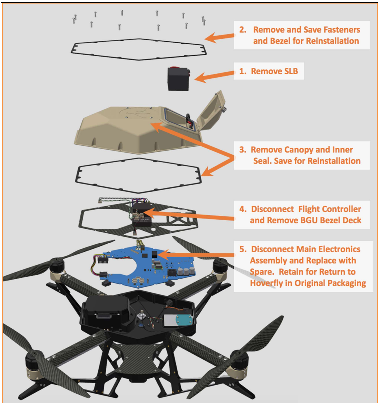
Figure 47. Main Electronics Assembly Replacement
