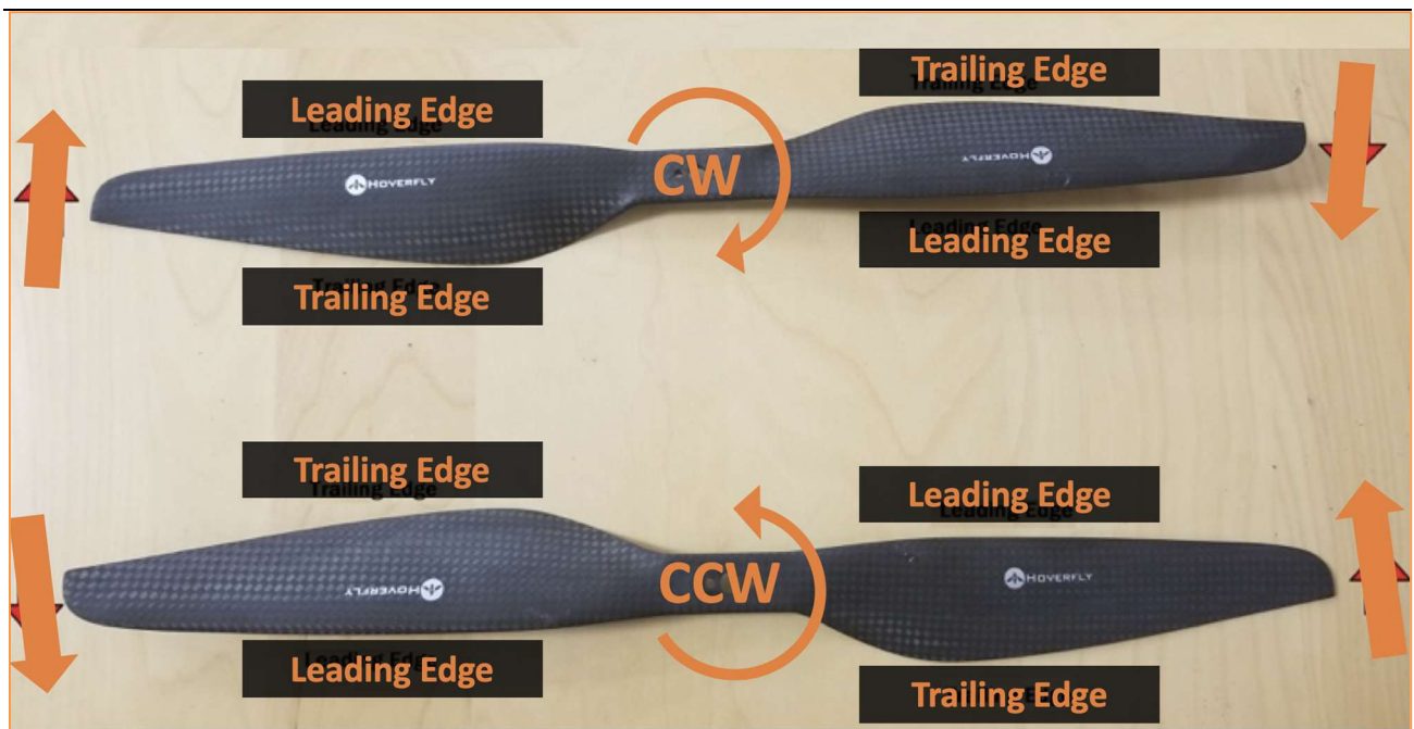
Figure 44. Propeller CW, CCW Shape Reference
