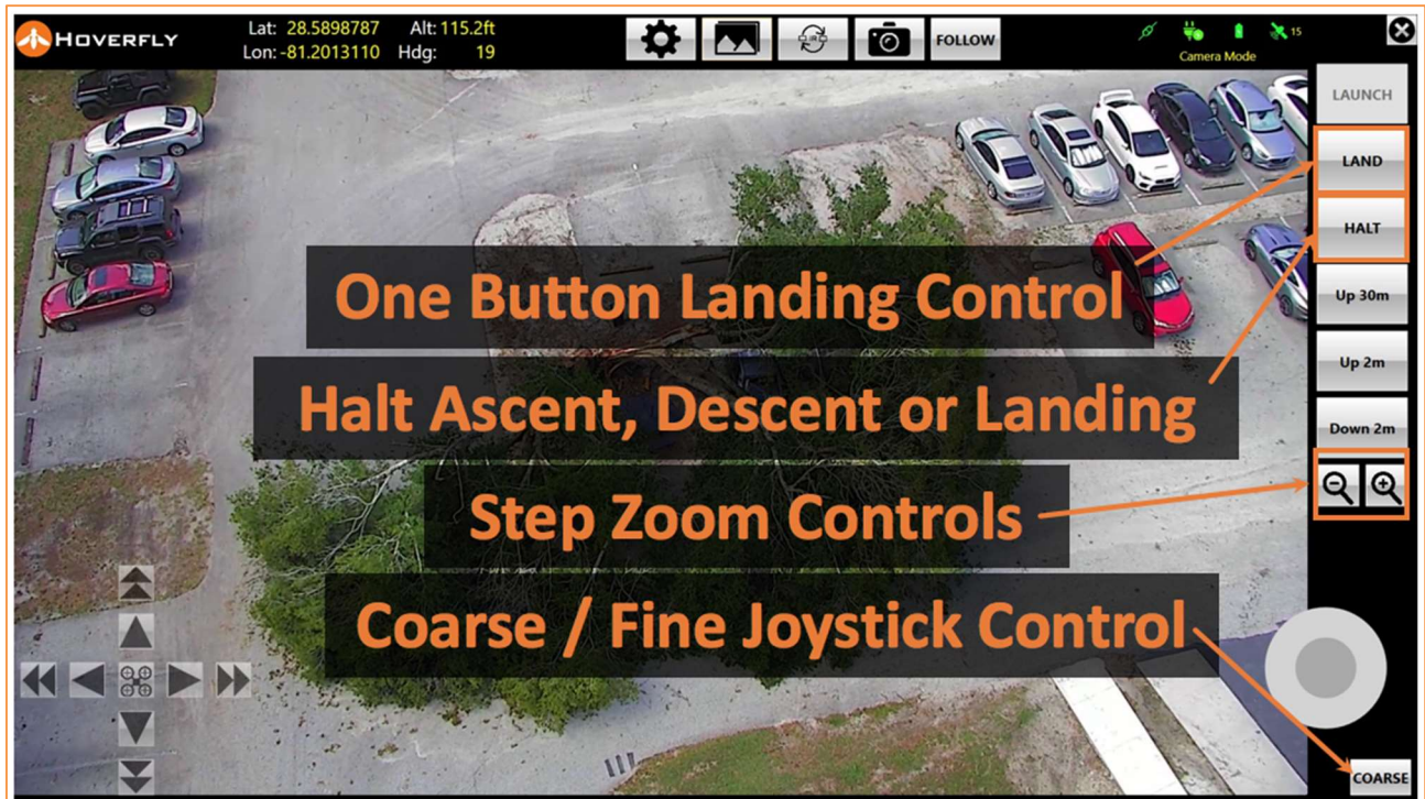
Figure 23. Flight and Sensor Controls Overview
