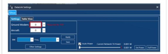
If this ID is not set, the Vector will fly without ToF data and navigation in GNSS denied mode which will be significantly more difficult.
