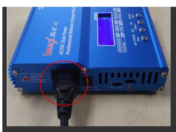
6. The SKYRC charger/discharger will power on and the message LiPo BALANCE CHG will appear on the display screen.
