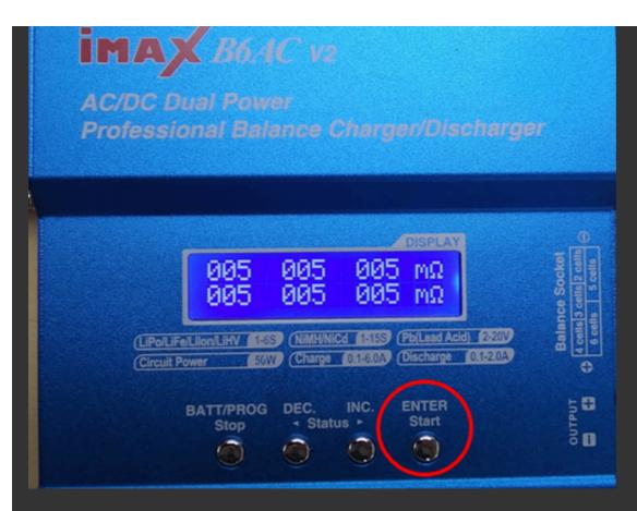
9. Verify the internal resistance of each cell.
