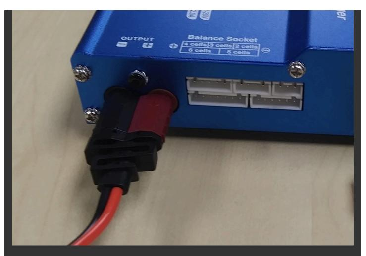
4. Connect the LiPo Balance Lead to the SKYRC charger/discharger.
