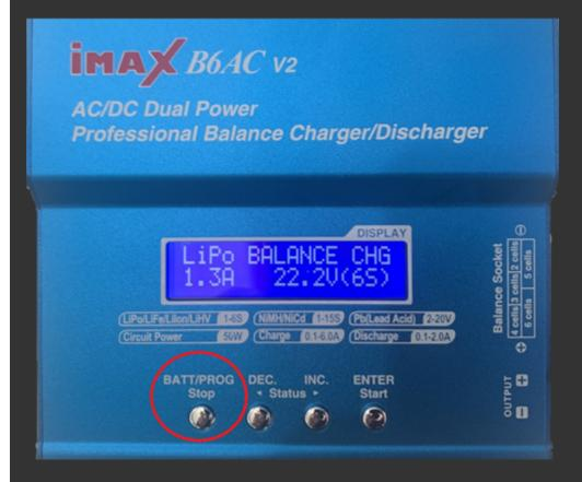
7. The BATT/PROGRAM screen with sub-menu will display. Press the DEC/Status button until the BATT RESISTANCE sub-menu appears.
