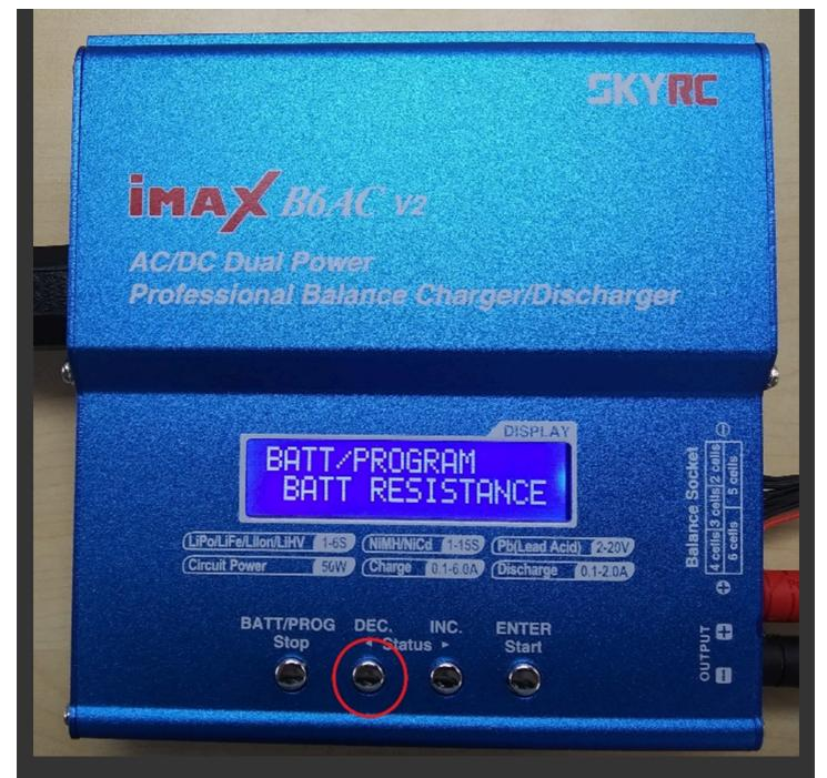
8. Press the ENTER/Start button. The m $\Omega$  reading for each battery cell is displayed.
