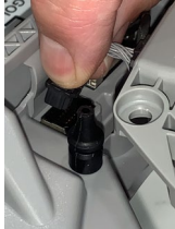
This side of the camera data connector faces the Hadron Camera.
