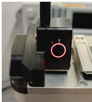
Figure 5 Charger connector pre-heat button
