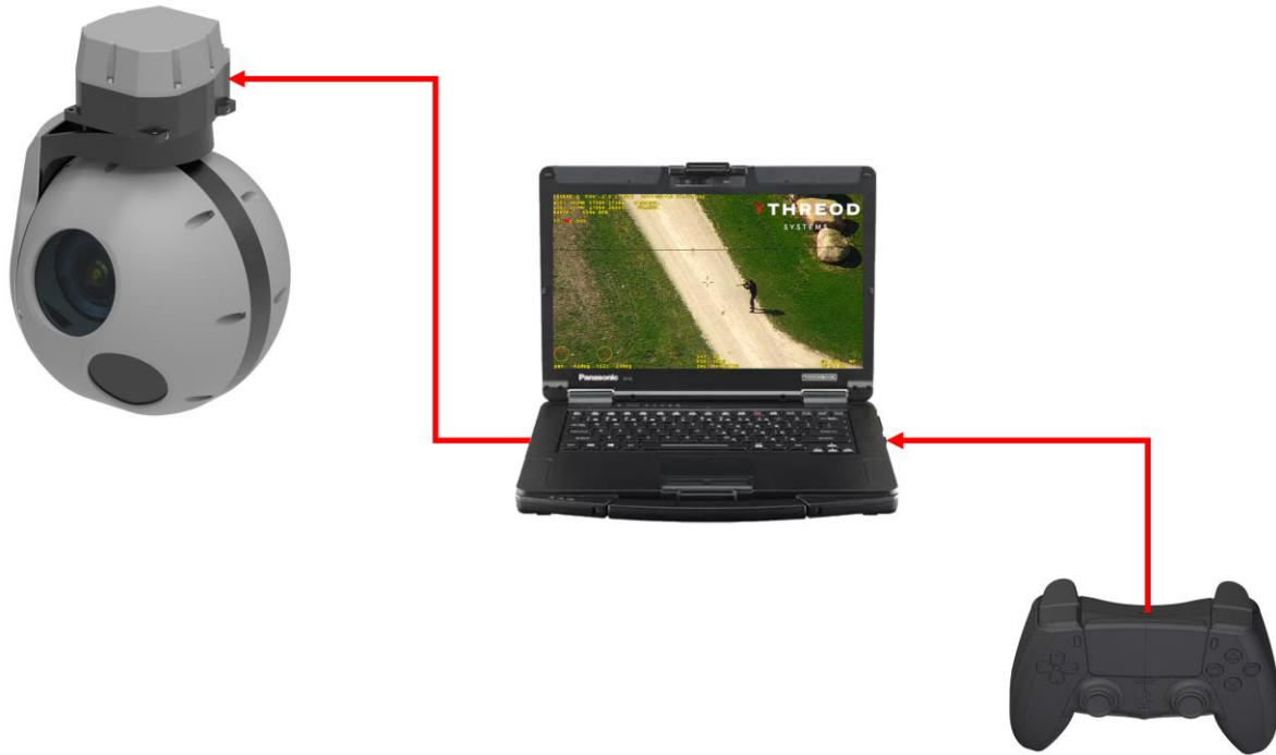
Figure 20: Mission software deployment – payload operator
