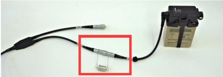
Figure 13. Power & comm cable connected to battery.
