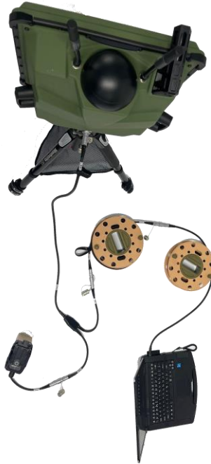
Figure 15. Ethernet extension cable connected to GCS.
