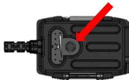
Figure 16. Powering on the battery.
