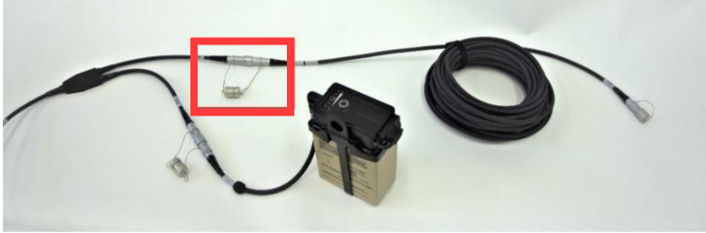
Figure 14. Power & comm cable connected to the ethernet extension cable.
