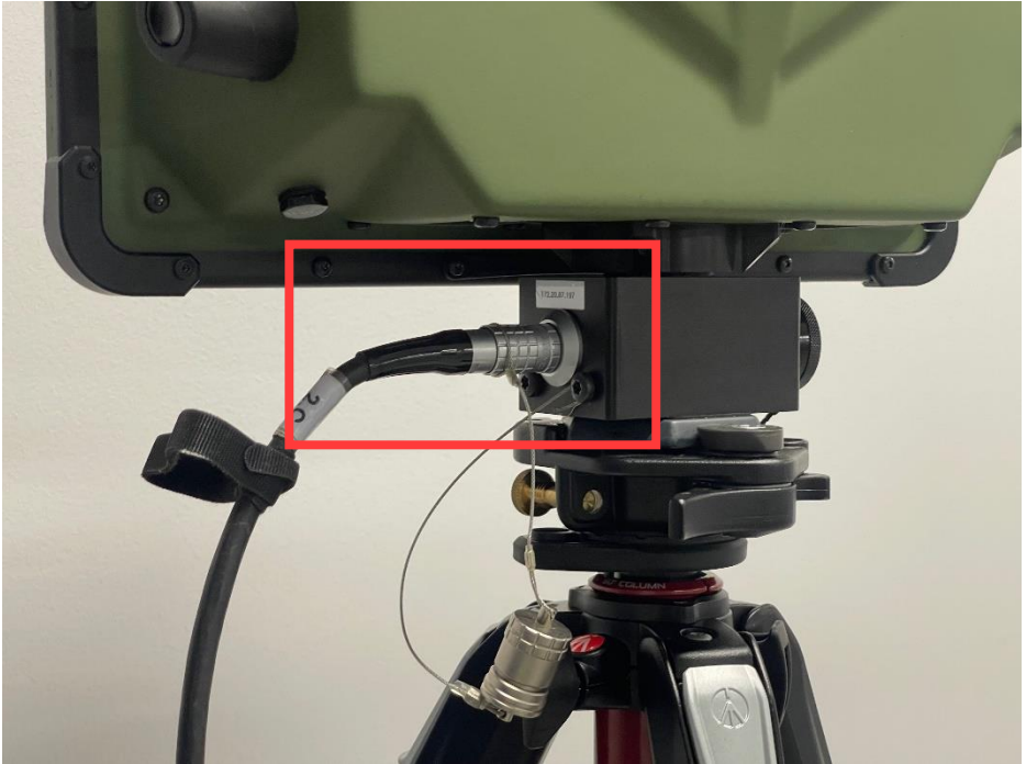
Figure 12. Power & comm cable connected to GDT 50P module.
