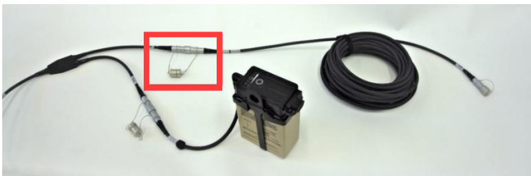
Figure 23 - Power & comm cable connected to ethernet extension cable.
