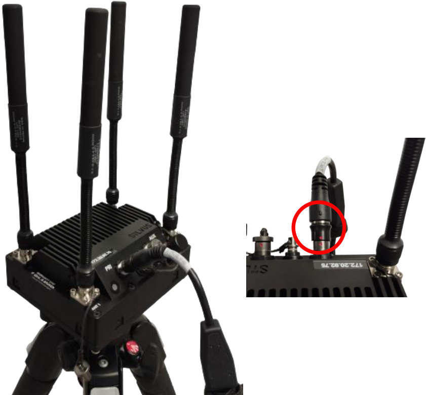
Figure 21 - Radio with antennas and data cable installed
