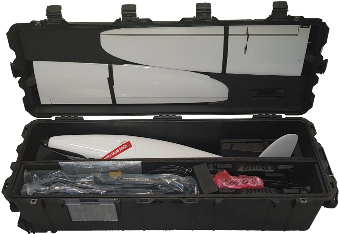
Picture: Example of complete Heidrun EO/IR UAS kit in a single flight case.
