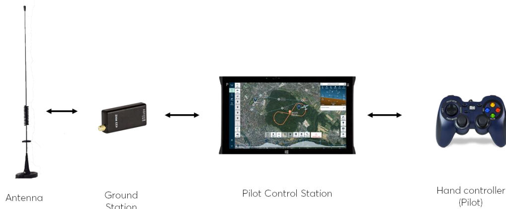
Picture: System diagram for Cumulus
