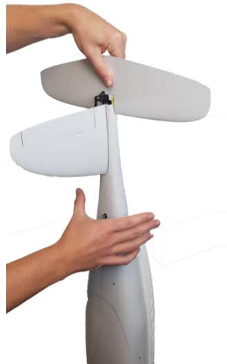
Picture: Check elevator mounting with caution
