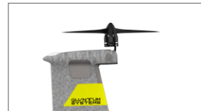
Rear alignment: tilted upwards correct for take-off/landing CORRECT
