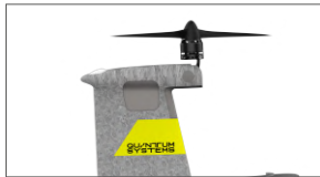
Rear alignment: tilted upwards CORRECT
