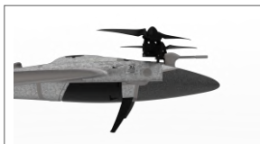
Front alignment: tilted upwards correct for take-off/landing CORRECT
