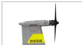
Rear alignment: neutral position correct for forward flight CORRECT
