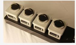
The lights on the side of the batteries show the battery level. The light representing the highest charge level blinks to indicate that the battery is charging.
