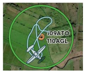
ATTENTION: The flight path is not optimized for looking at objects inside the flight area. To loiter around an object of interest, use the circular loiter pattern or the camera cruise mode.
