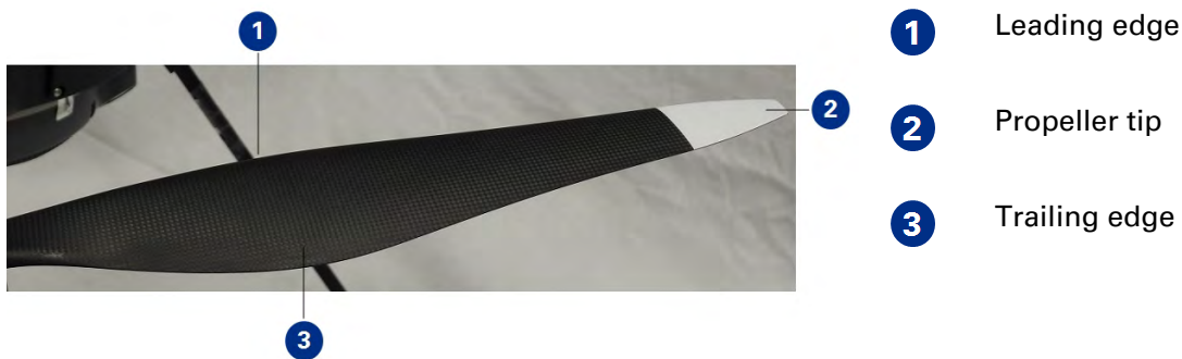
Propeller inspection locations
