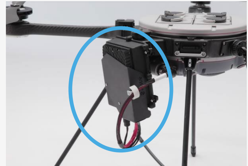
Air module, providing data over tether, connected to Bk2 Power/Ethernet port
