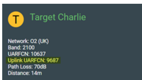
Fig 217. UMTS Hold – uplink UARFCN
