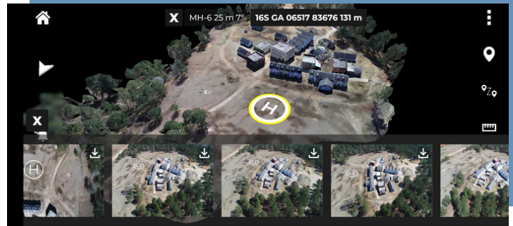
Figure 13: The user is analyzing the raw media images of an HLZ. The landing zone is marked in all the raw images.
