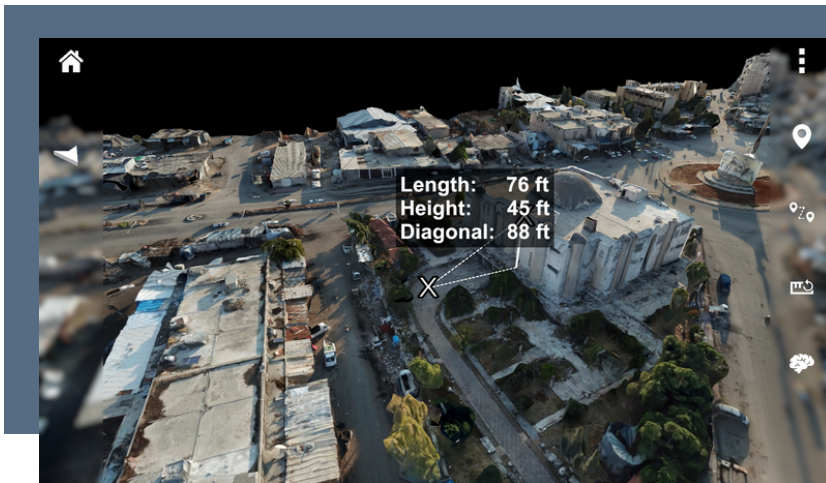
Fig 10: Using the AI Measurement Tool, Farsight measures the length, height, and diagonal from a specific point.
