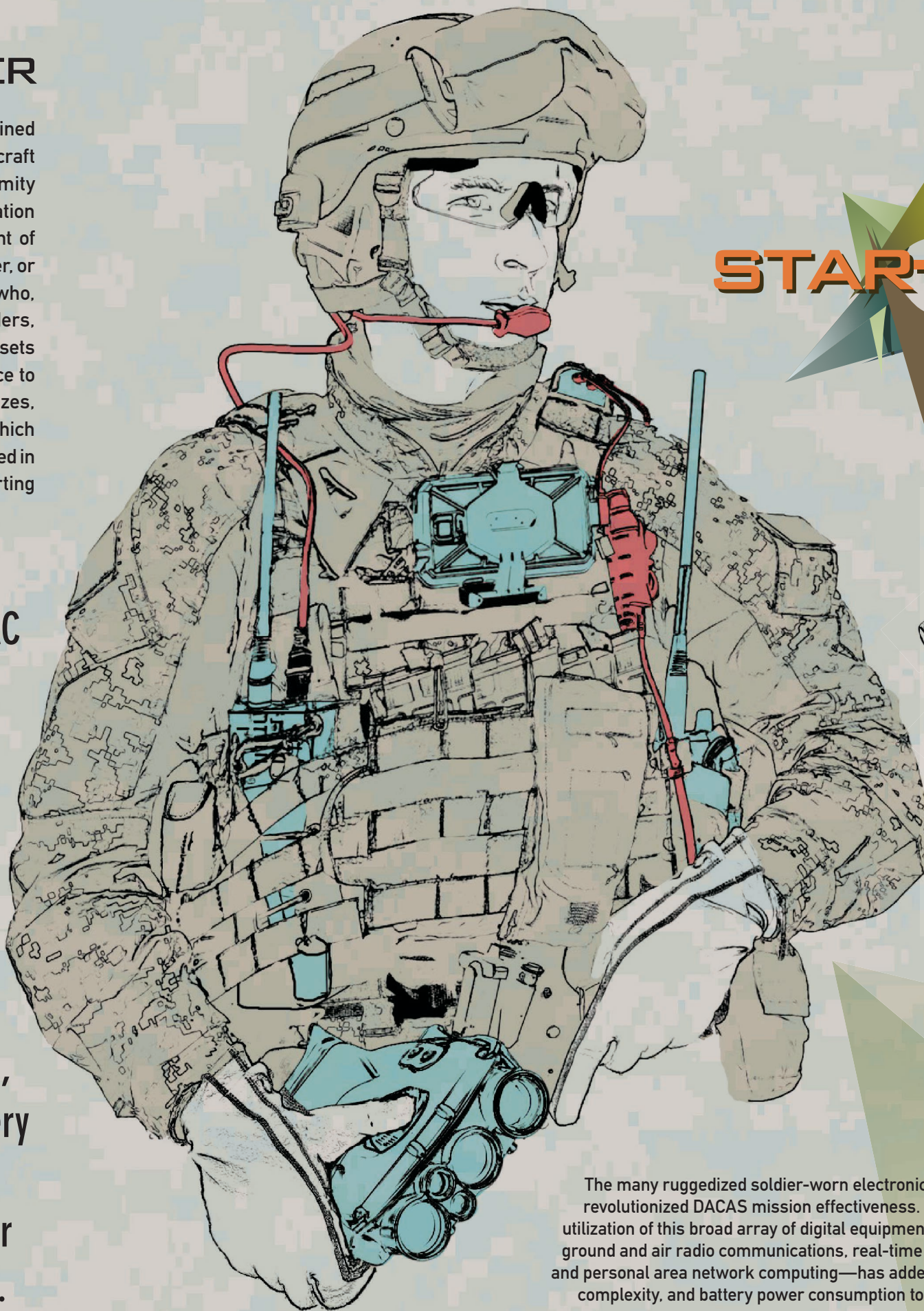
Dismounted soldier C4ISR technologies integrated on vest and interconnected with NATO STANAG 4695 / Nett Warrior connectors and cables (Glenair Mighty Mouse 807)
