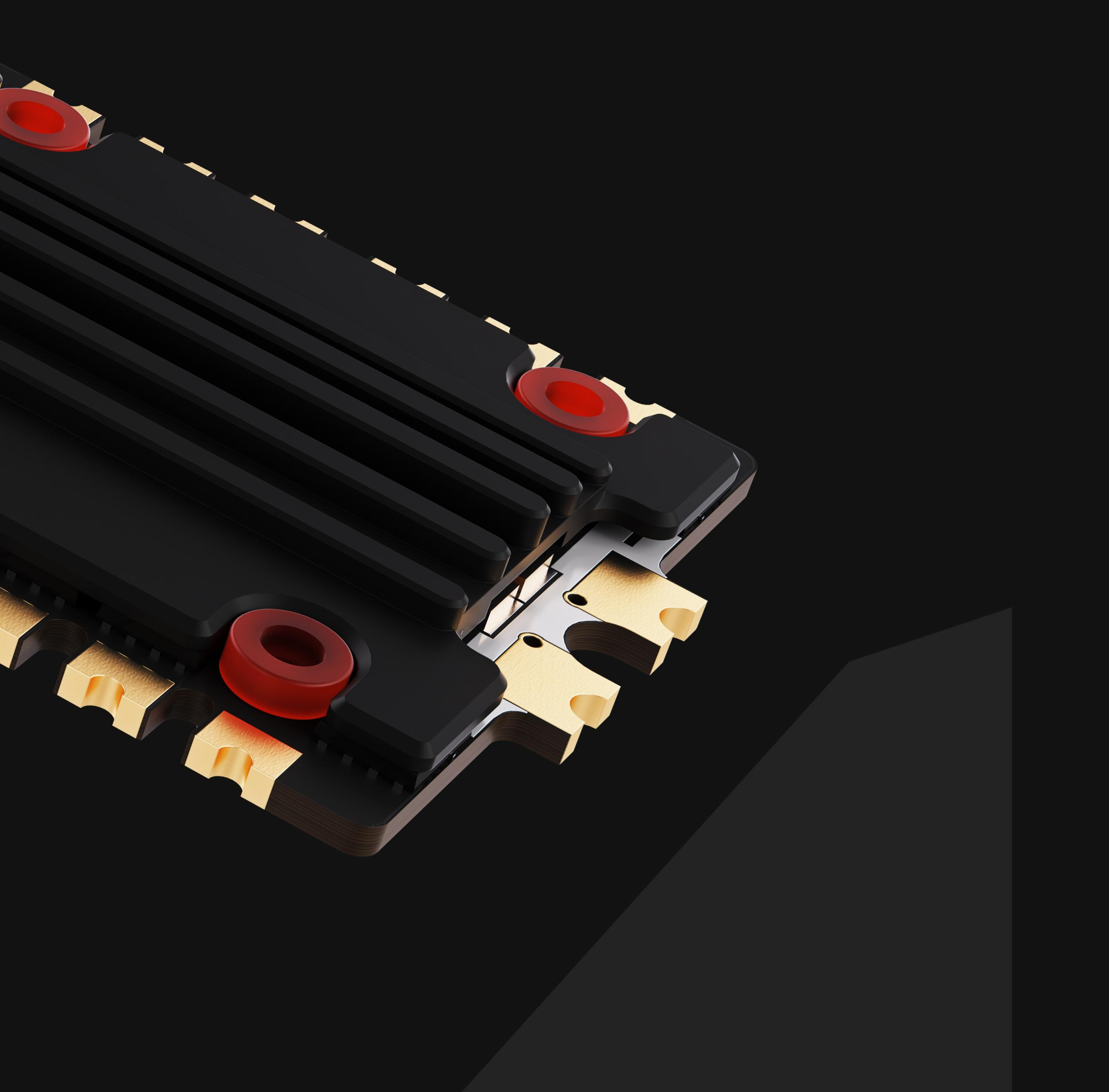
Robust 70A BLHeli-32 4-in-1 ESC, with BL-Heli 32, Bidirectional DShot, for 30x30 mounting.
